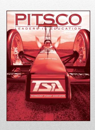
Students design and construct a CO2 powered dragster to meet specific regulations. Overall score includes wind tunnel test score, appearance, meeting specifications, drawing and speed points.
